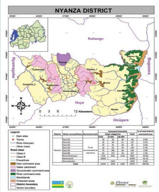
Figure 44: Potential irrigation water source
