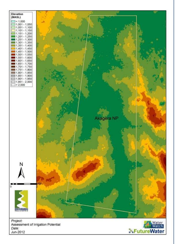
Figure 64: DEM Akagera NP focal area. Resolution 1 arc second (+/- 30m). (Source: ASTER).
