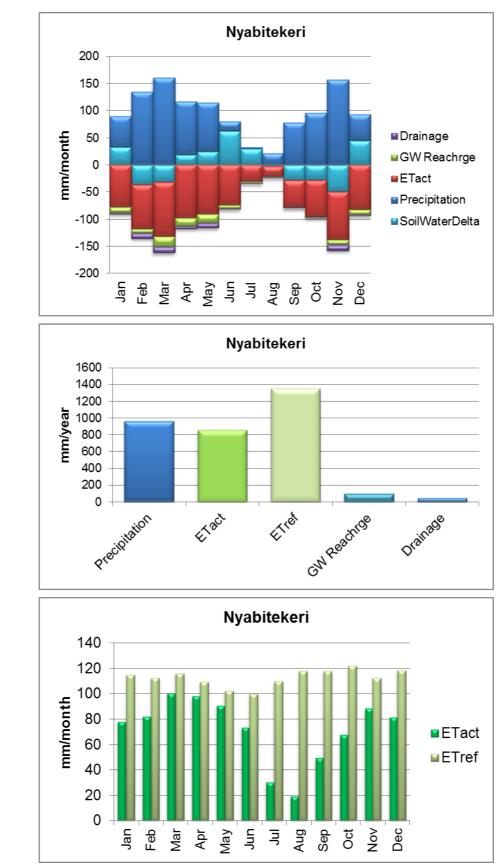
Figure 83: Water balances for the area based on the high resolution data and modeling approach for Nyabitekeri focal area. (Source: NELmod).
