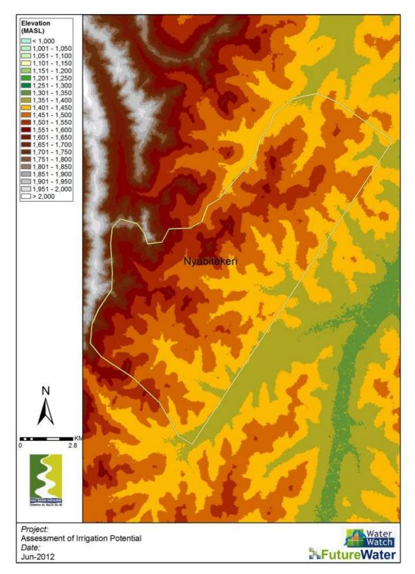
Figure 78: DEM Nyabitekeri focal area. Resolution 1 arc second (+/- 30m). (Source: ASTER).
