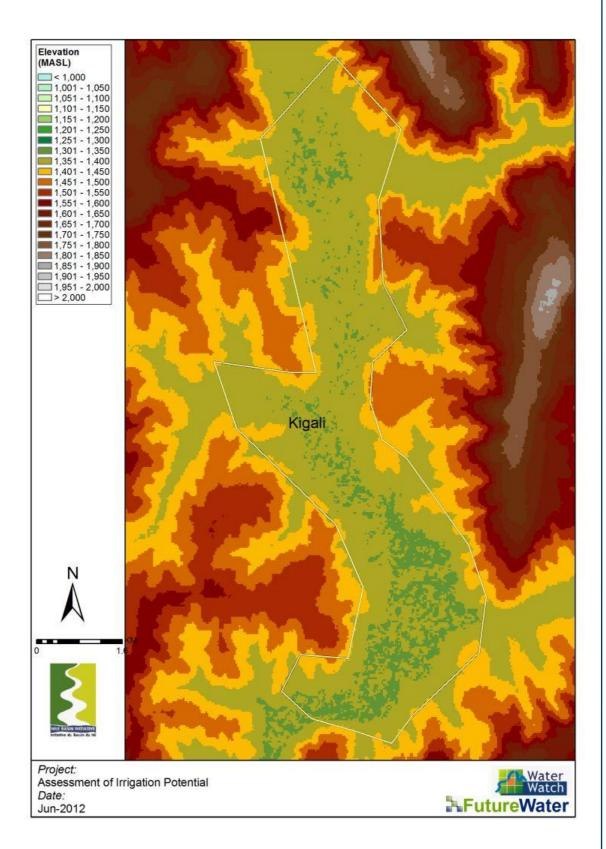
Figure 92: DEM Kigali focal area. Resolution 1 arc second (+/- 30m). (Source: ASTER).
