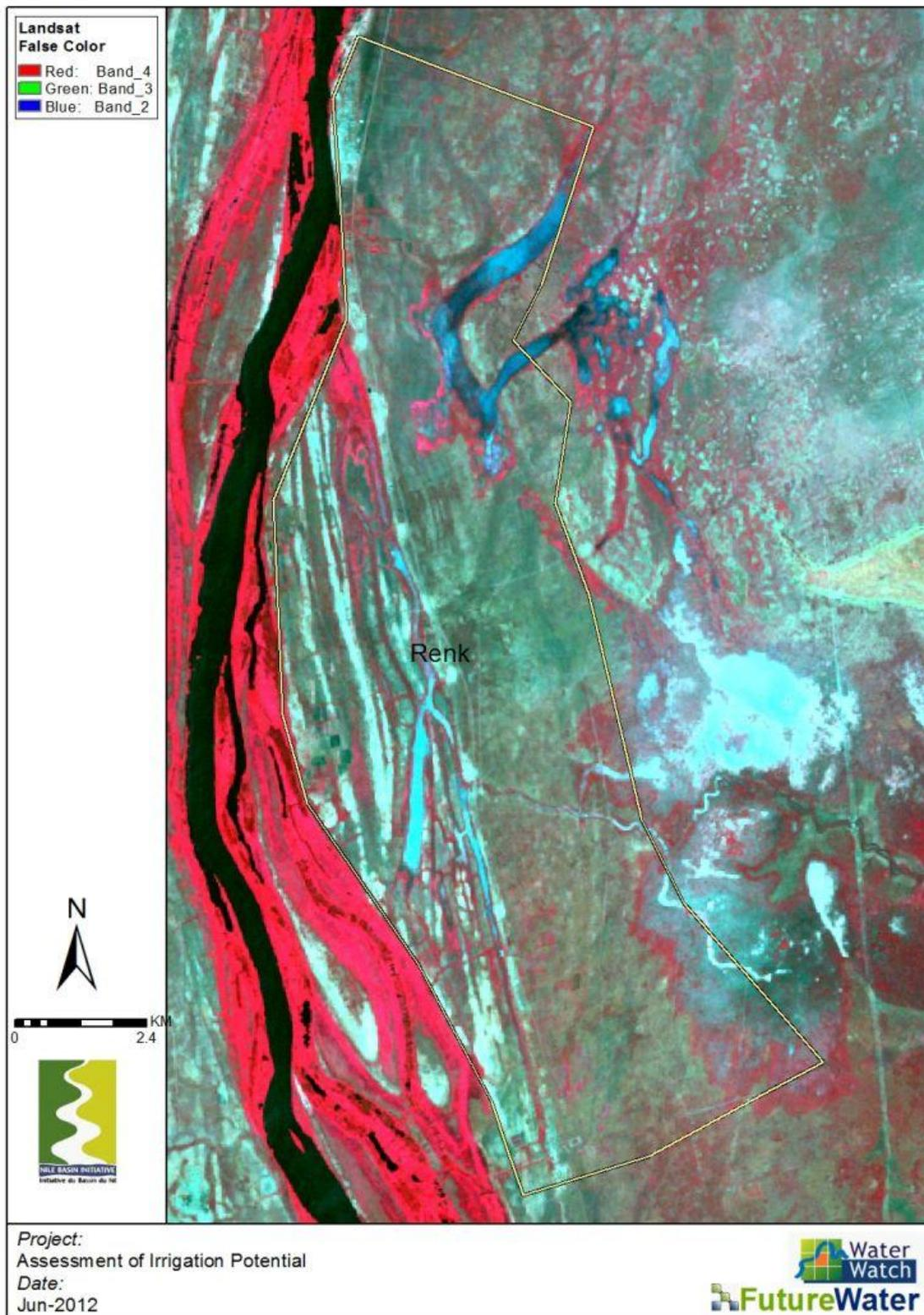
Figure 96: Landsat False Color Composite indicating current productivity of Renk focal area.
