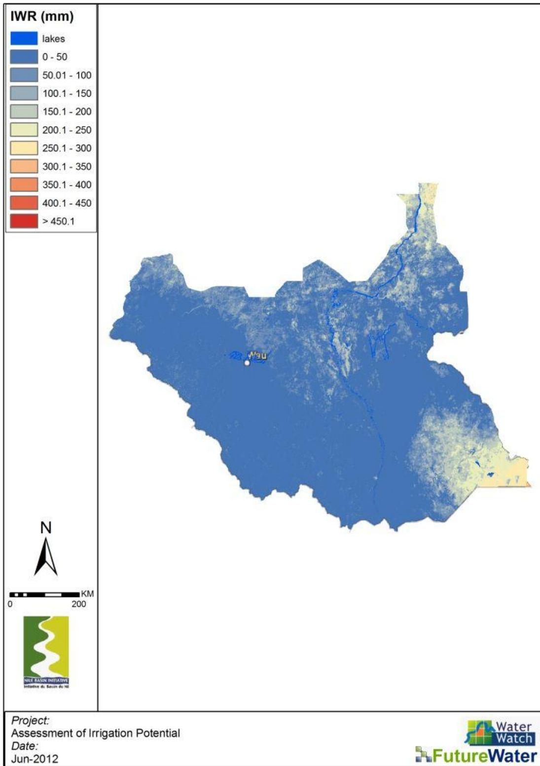
Figure 12: Reference evapotranspiration (top), actual evapotranspiration (middle), and irrigation water requirement (bottom) for August (Average 2001-2010). (Source: study analysis).
