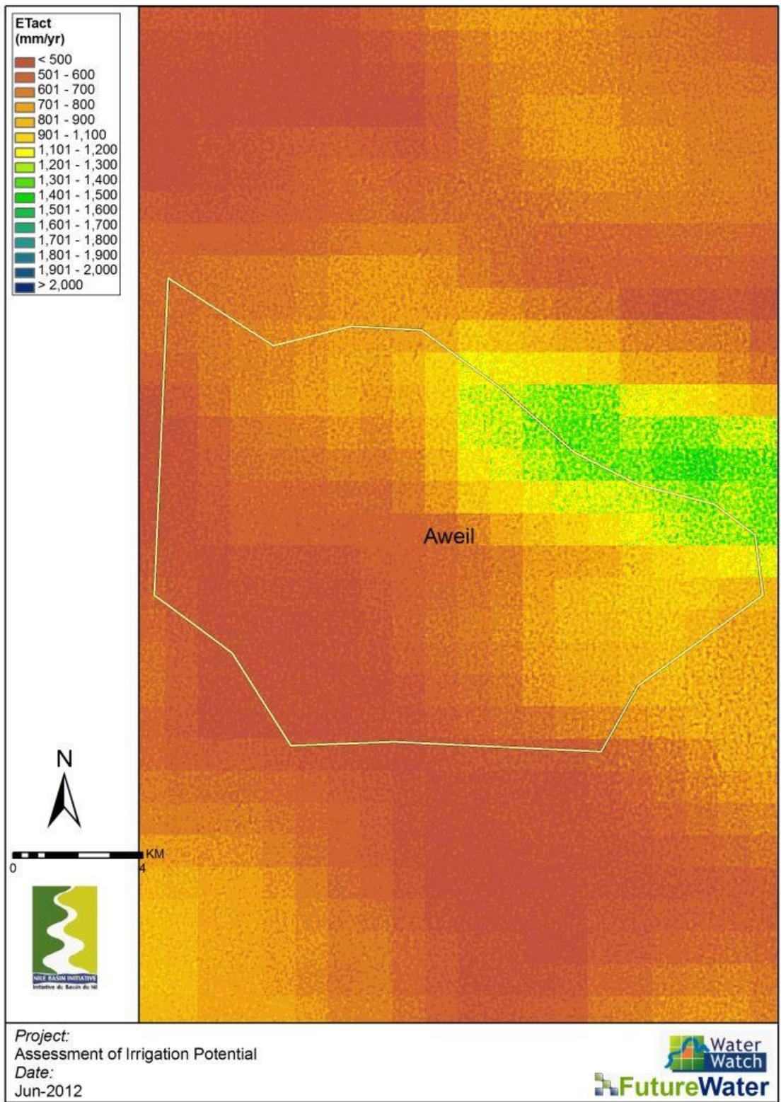
Figure 76: Water balances for the area based on the high resolution data and modeling approach for Aweil focal area.
