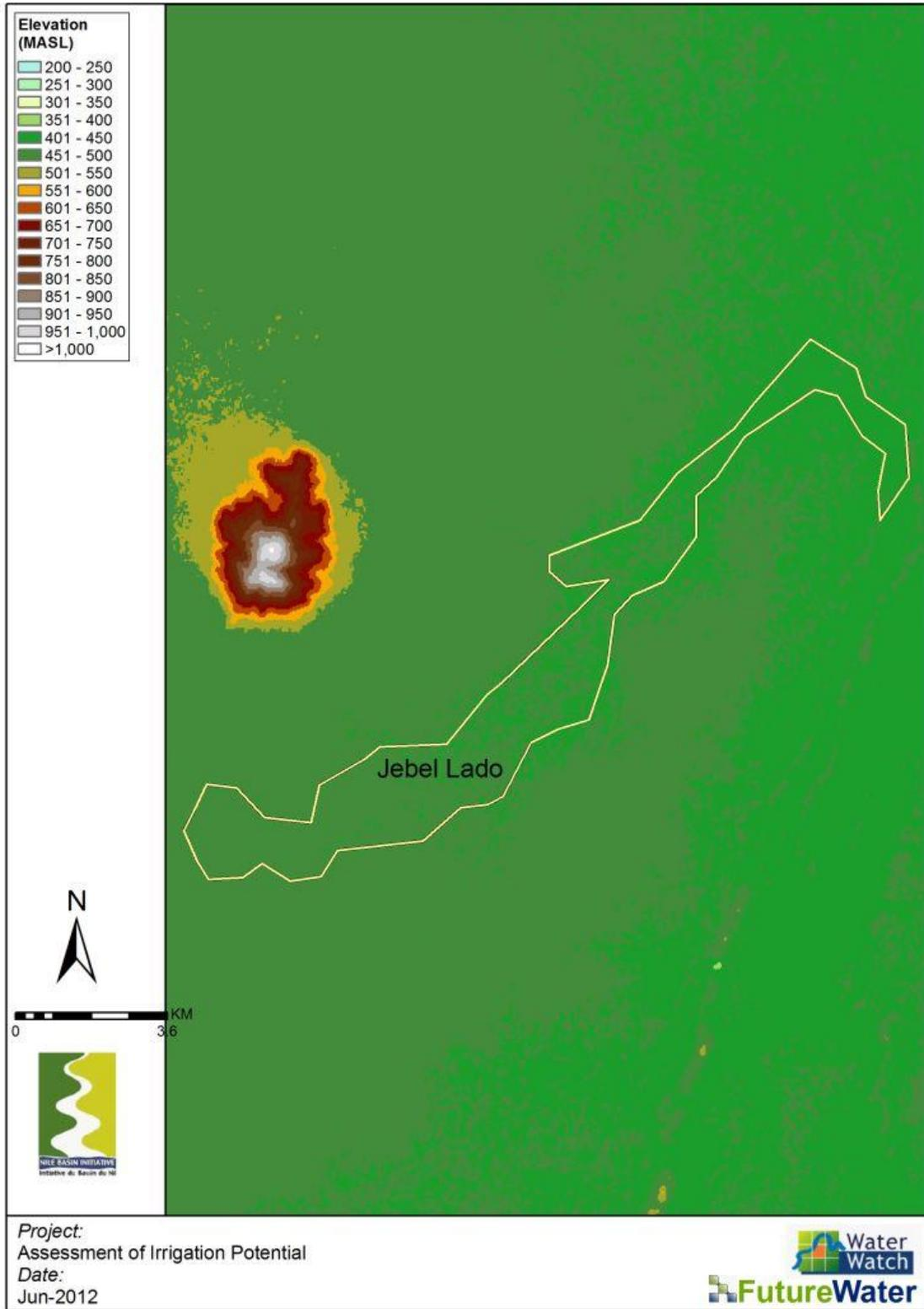
Figure 33: DEM Jebel Lado focal area. Resolution 1 arc second (+/- 30m).
