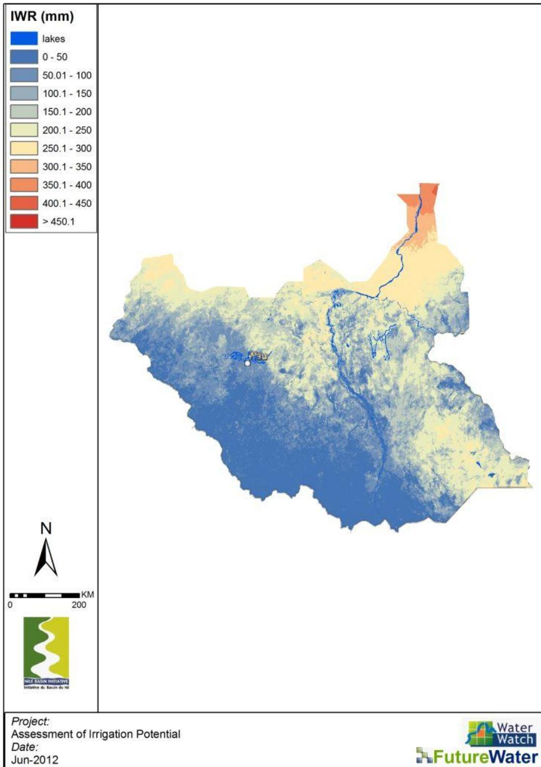
Figure 10: Reference evapotranspiration (top), actual evapotranspiration (middle), and irrigation water requirement (bottom). For June (Average 2001-2010). (Source: study analysis).
