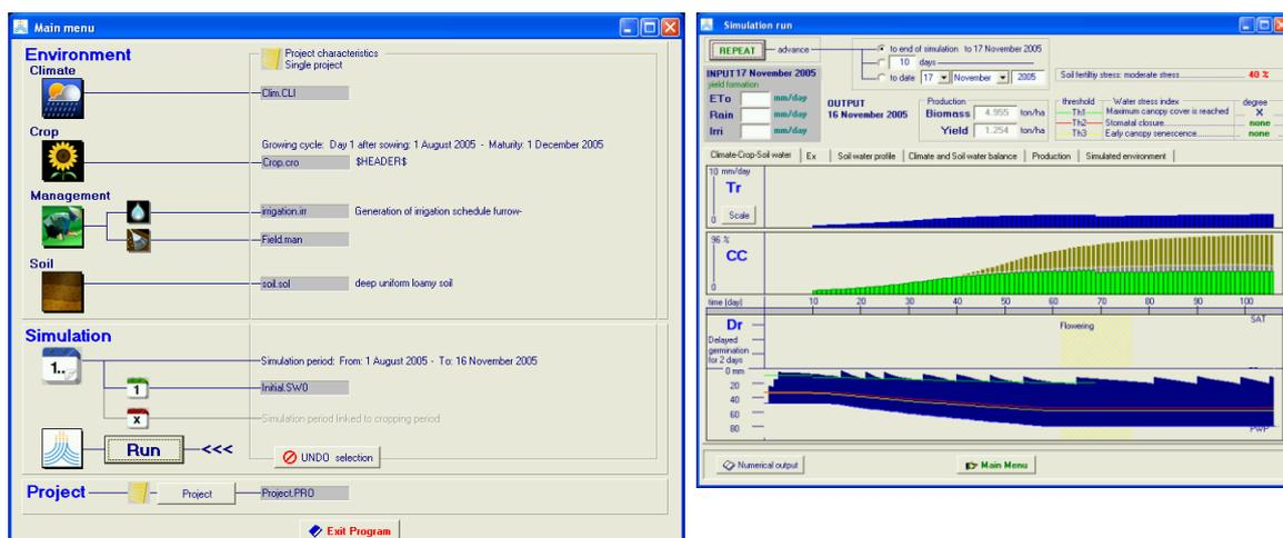
Figure 44: Typical example of AquaCrop input and output screens.
