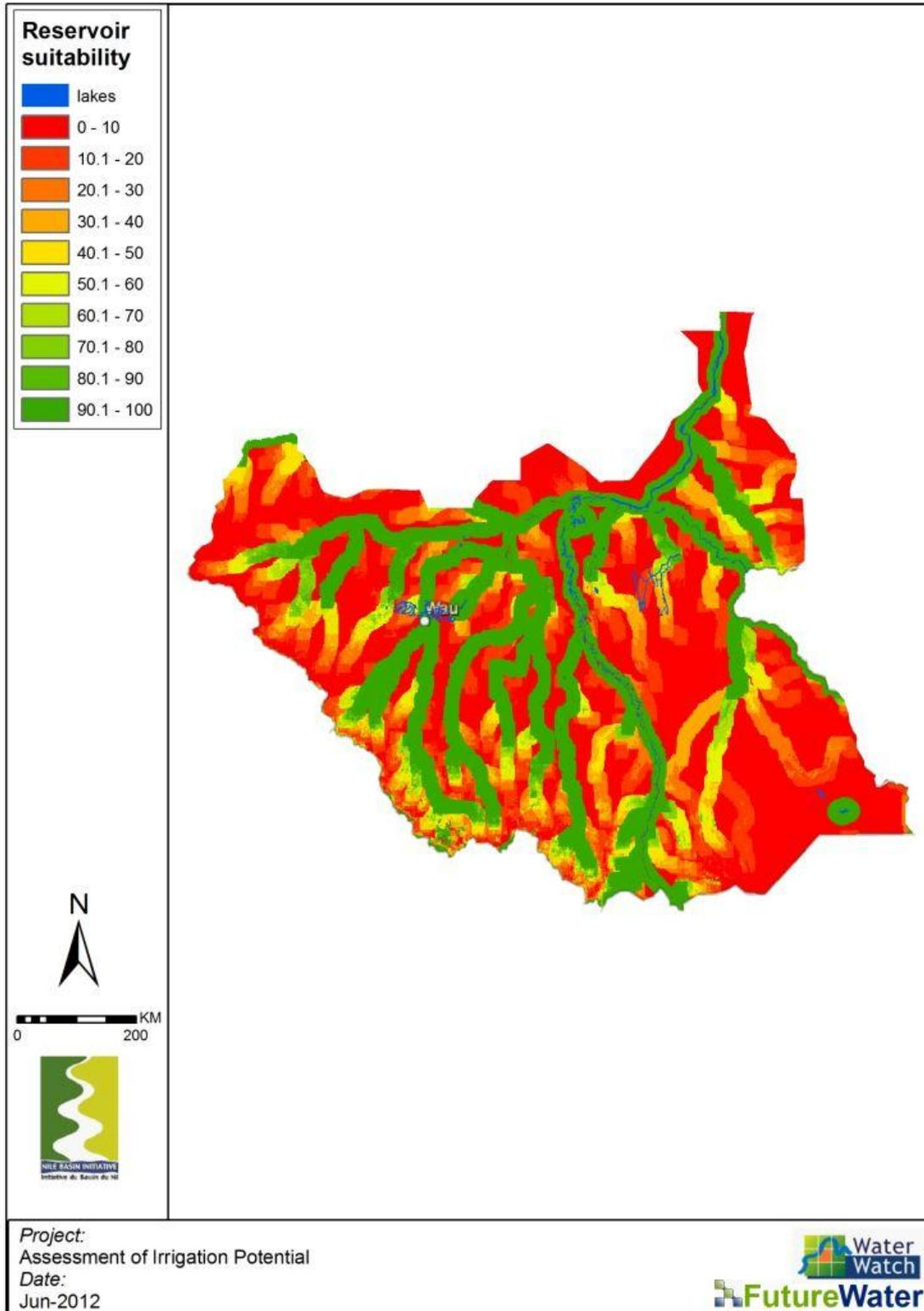
**Figure 17. Water availability for irrigation. Total coverage (top), coverage from surface water (second), coverage from ground water (third), and from potential reservoirs (bottom). (Source: study analysis).**
