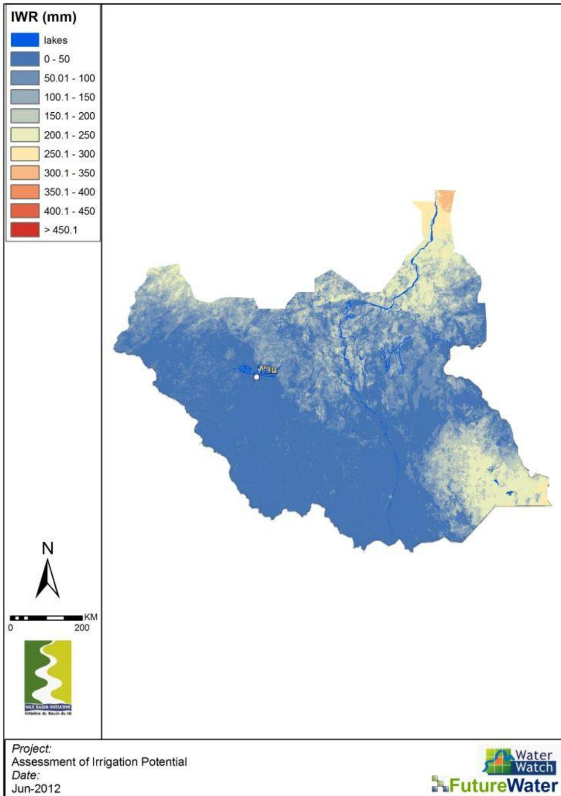
Figure 11: Reference evapotranspiration (top), actual evapotranspiration (middle), and irrigation water requirement (bottom) for July (Average 2001-2010). (Source: study analysis).
