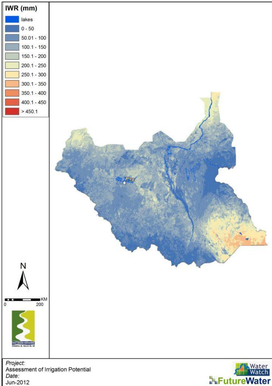
Figure 15: Reference evapotranspiration (top), actual evapotranspiration (middle), and irrigation water requirement (bottom) for November (Average 2001-2010). (Source: study analysis).
