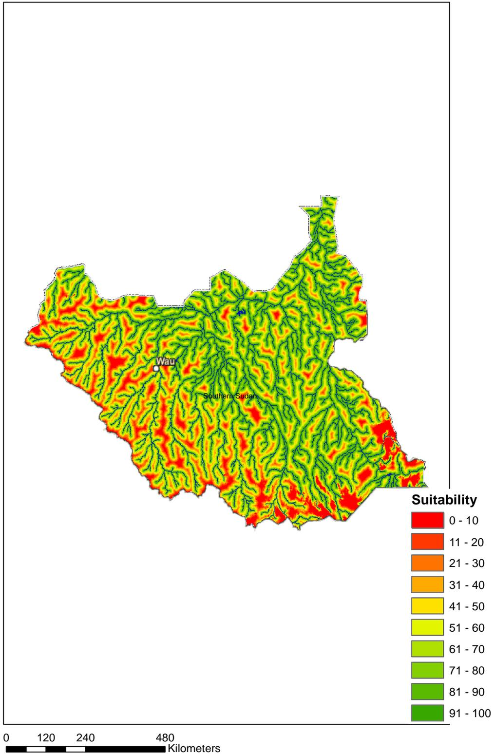
**Figure20: Average distance to a natural stream, lake or reservoir (top left), elevation above natural stream, lake or reservoir (top right), and access to water suitability score (bottom).**
