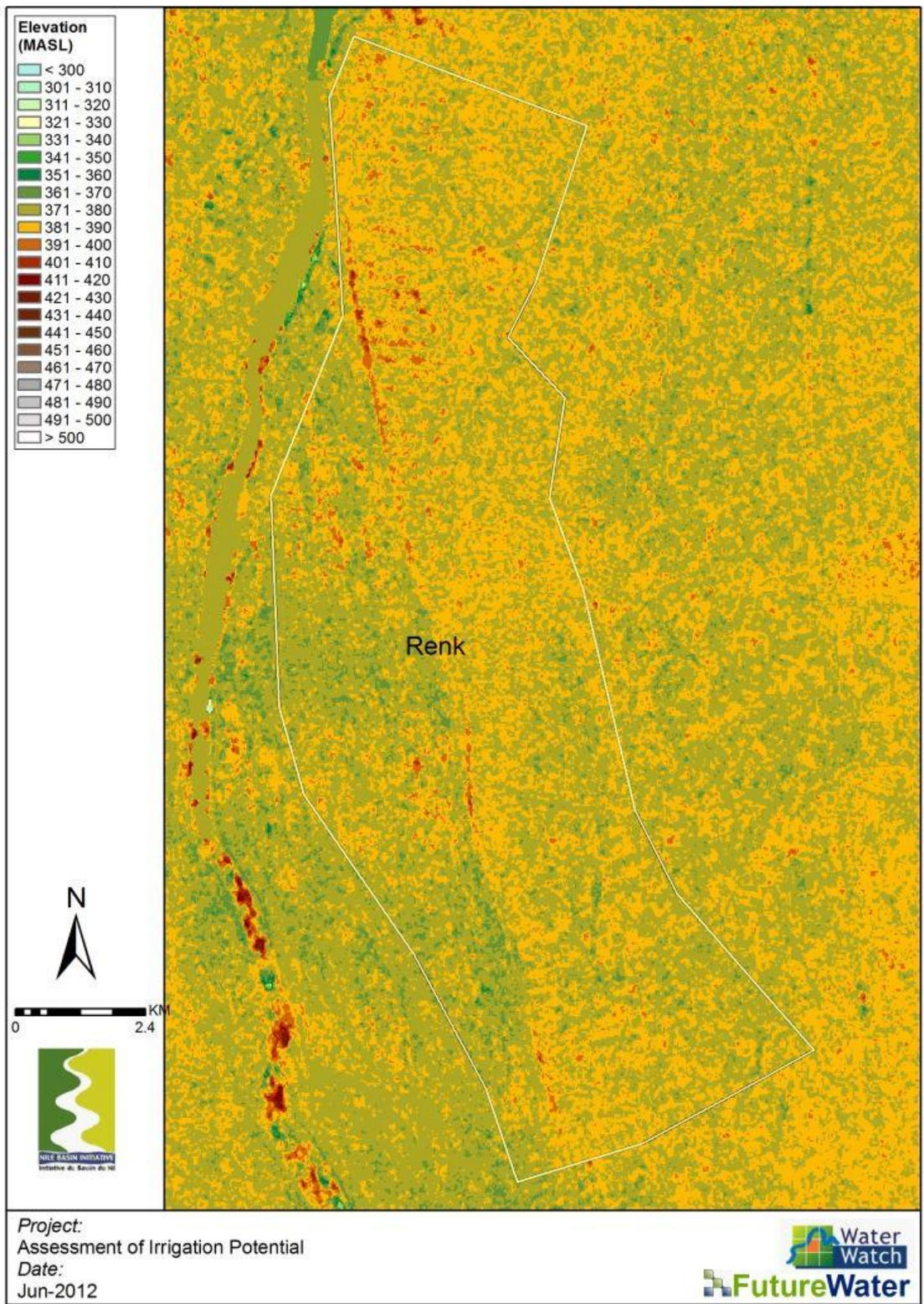
Figure 83: DEM Renk focal area. Resolution 1 arc second (+/- 30m).
