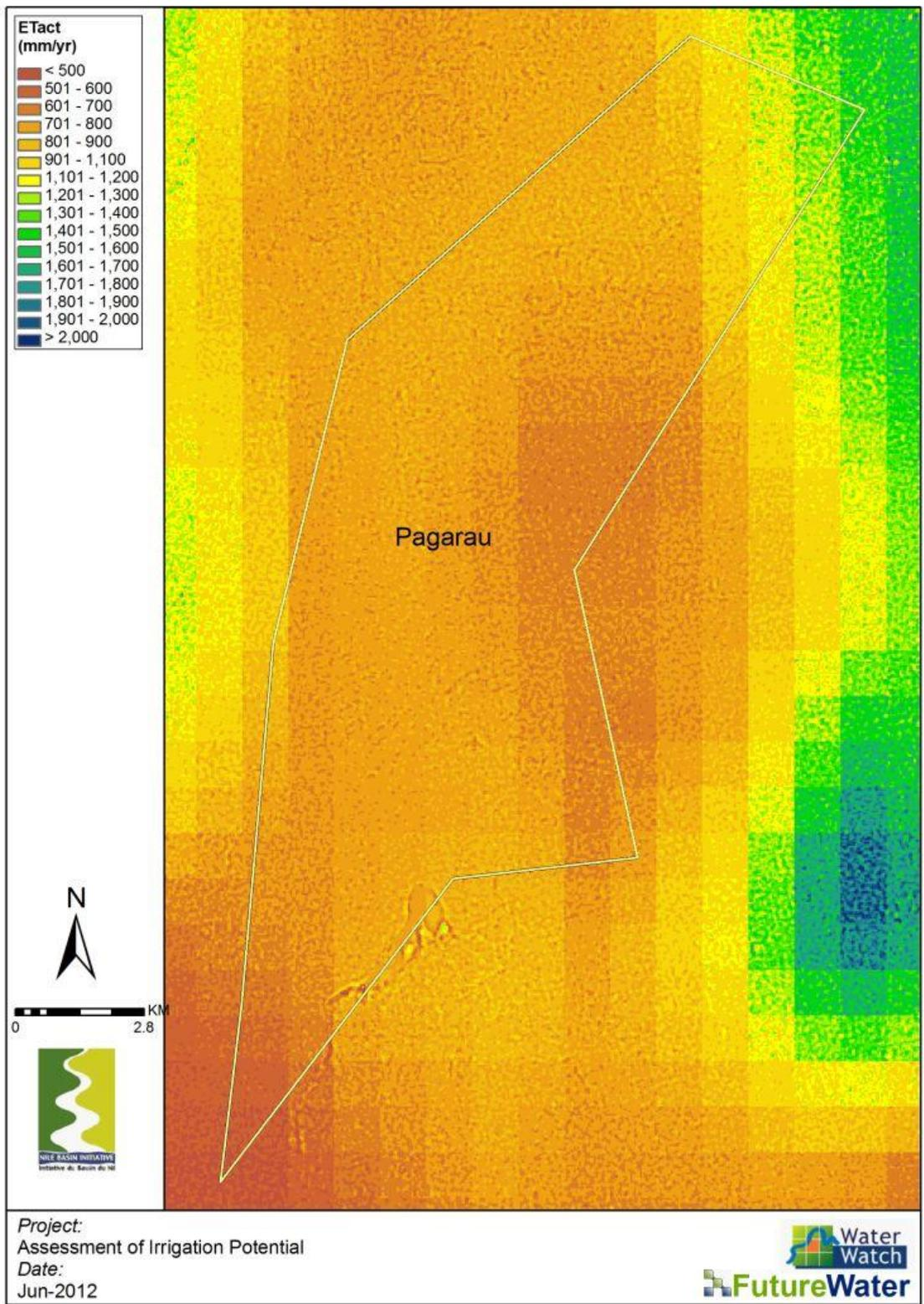
**Figure 58: Water balances for the area based on the high resolution data and modeling approach for Pagarau focal area.**
