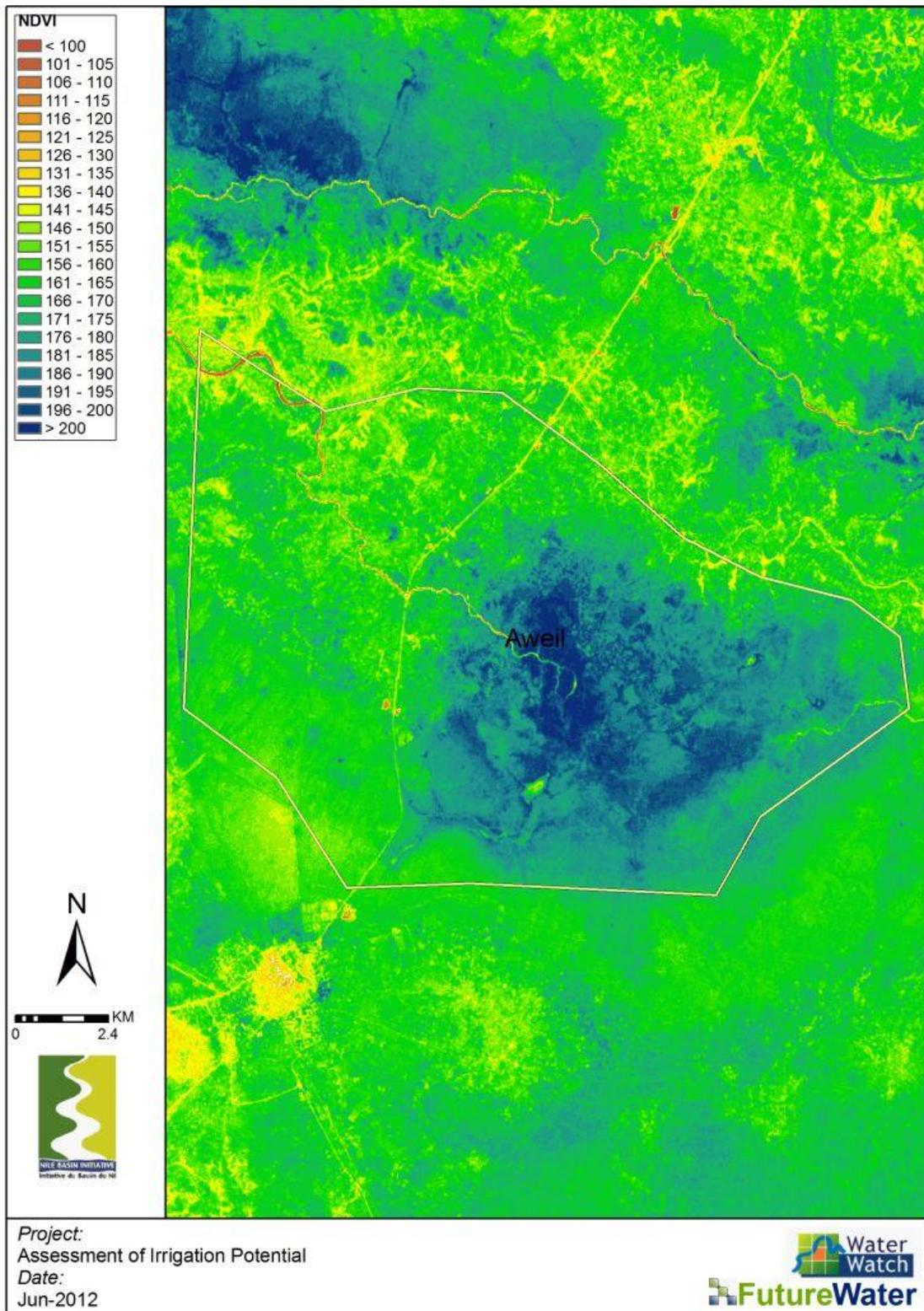
Figure 69: High resolution NDVI for Aweil focal area
