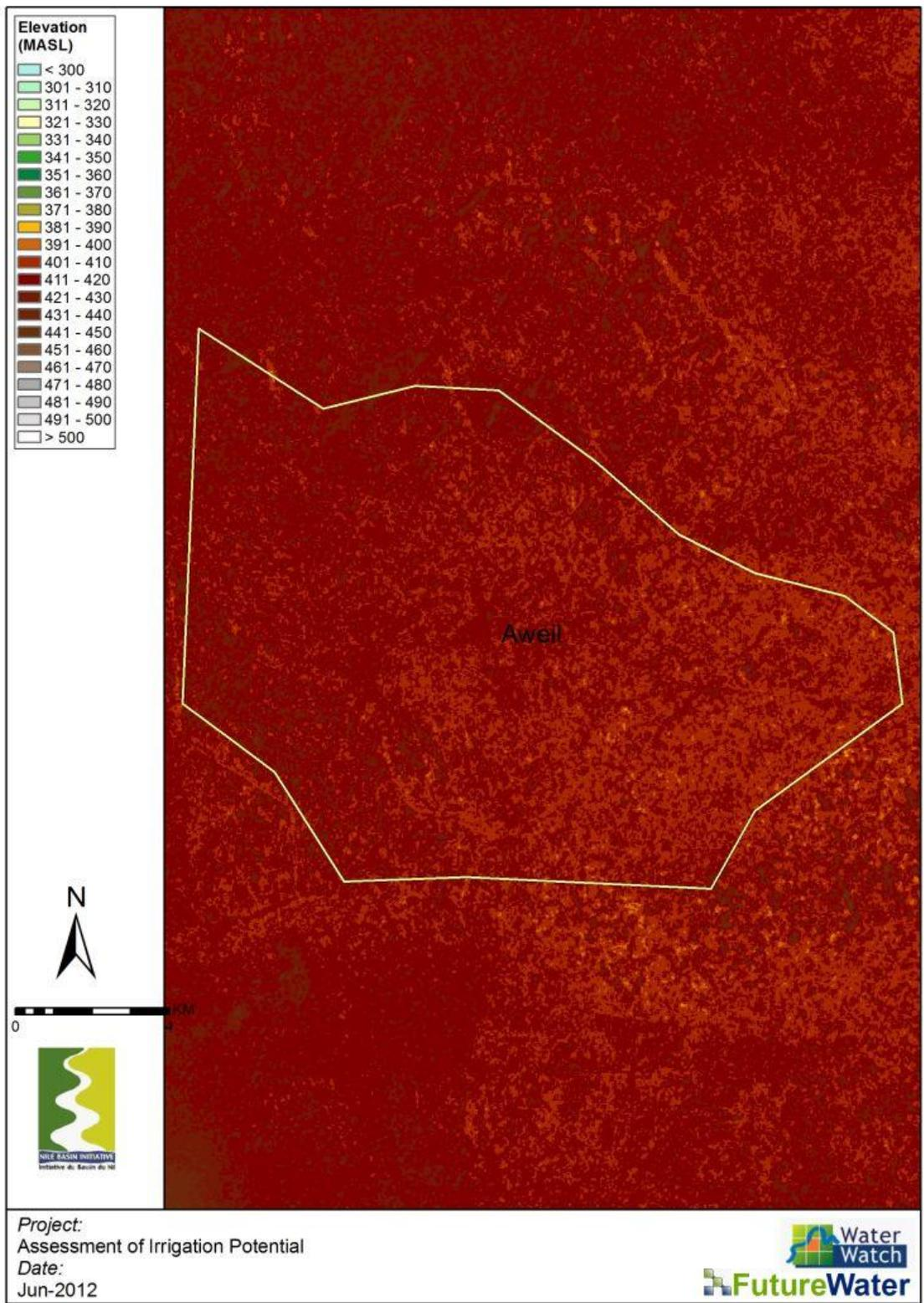
Figure 66: DEM Aweil focal area. Resolution 1 arc second (+/- 30m).
