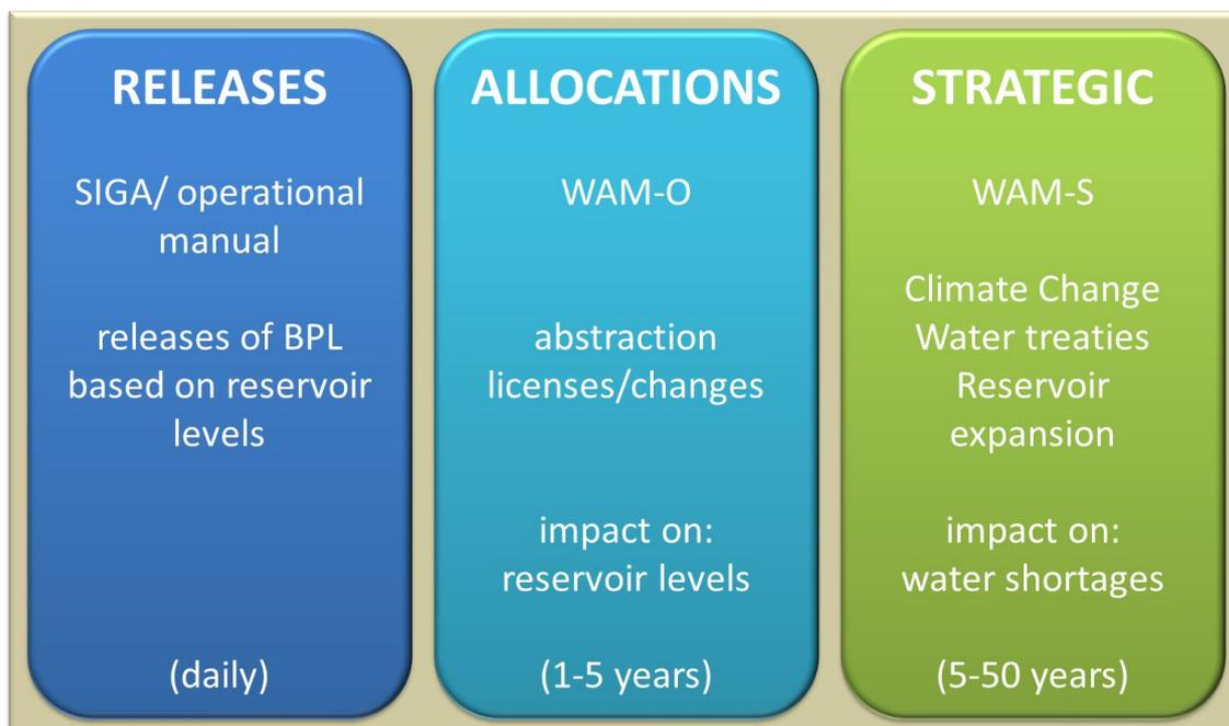
**Figure 5. The three tools to support decision making for the Umbeluzi basin.**
